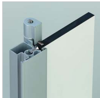
HPL door with door stop profile – hinges screwed hidden from sight
